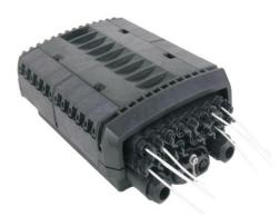
The FAT outdoor fiber access terminal is able to hold up to 16 subscribers and 96 splicing points as closure. It's used as a splicing closure and a termination point for the feeder cable to connect with the drop cable in FTTx network system. It integrates fiber splicing, splitting, distribution, storage and cable connection in one solid proteciton box.
